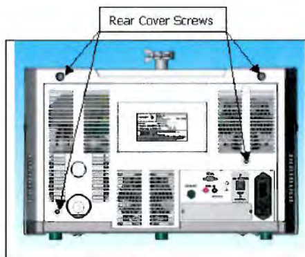
Figure 1-4 Location of Rear Cover Screws
