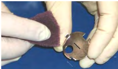
Figure 3-17 Cleaning the Ground Slit Plate
