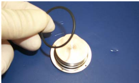
Figure 4-18 Removing the O-ring from Magnetic Pole Piece
