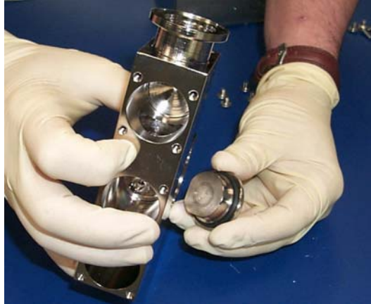
Figure 4-19 Removing the Second Magnetic Pole Piece
