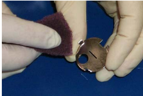
Figure 4-20 Discolored Ground Slit Plate
