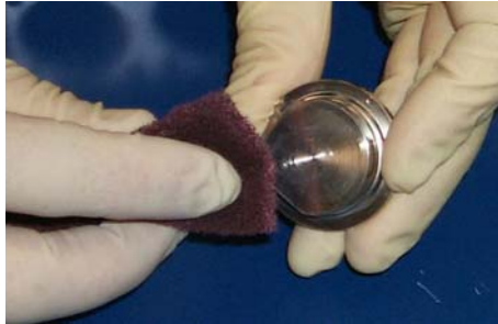
Figure 4-21 Discolored Ground Magnet Pole Piece
